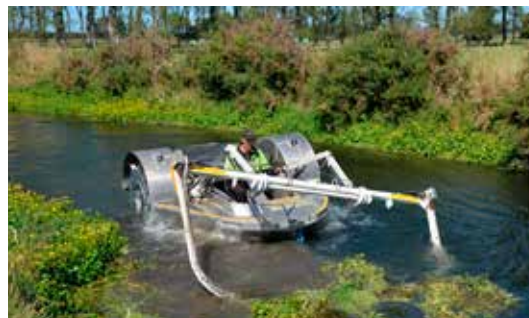
The weed cutter boat operating in the deeper Ararira River mainstem removes submerged macrophytes such as Elodea and Potamogeton crispus (both introduced species) along with emergent marginal species including monkey musk and watercress. After being cut with the weed cutter boat, macrophytes drift downstream to a site around 1.5 km upstream of the river mouth where they are captured by screens, removed from the river with a digger, and left to decompose.
