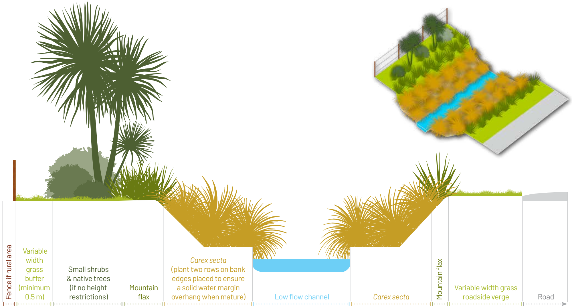
Cross section showing the profile of a typical two-stage channel with riparian planting.
