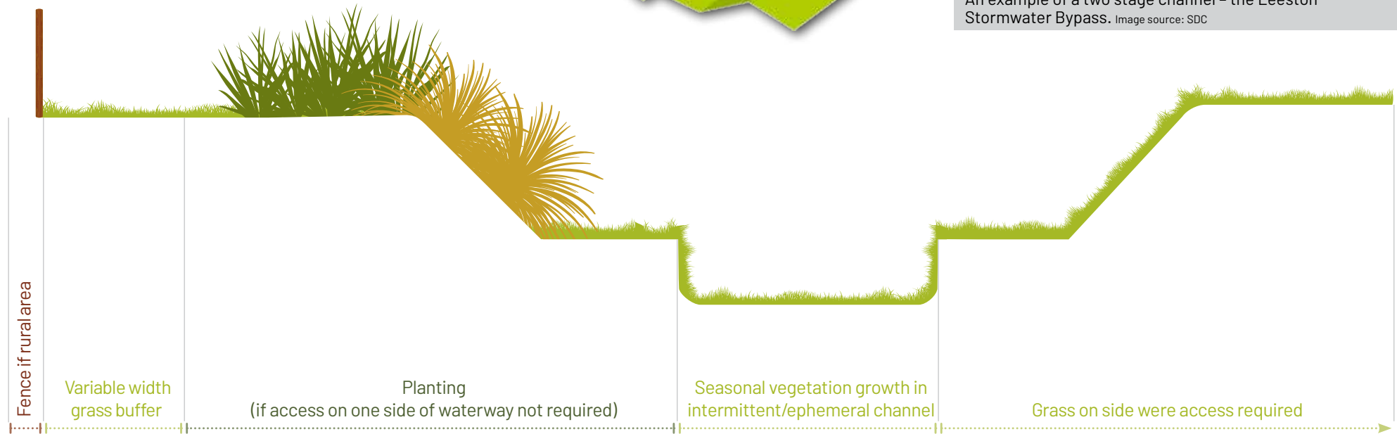
Cross section showing the profile of a typical two-stage channel with grass. Image source: EOS Ecology
